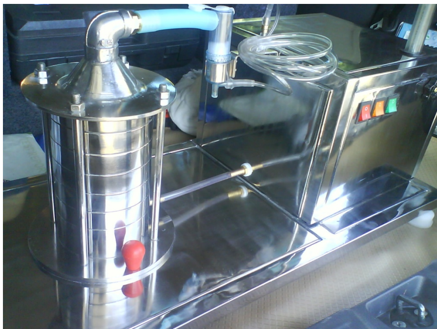
SITRA's Bacterial Filtration Efficiency Tester
